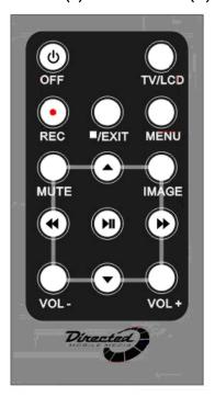
**NOTE:** This remote control does not function if the unit is docked in a overhead video unit. Use the overhead console's remote.
